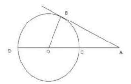
AB = 15 cm, AC = 7.5 cm Let 'r' be the radius of the circle. ∴ OC = OB = r AO = AC + OC = 7.5 + r In △AOB, AO<sup>2</sup> = AB<sup>2</sup> + OB<sup>2</sup>  $(7.5 + r)^2 = 15^2 + r^2$   $\Rightarrow \left(\frac{15 + 2r}{2}\right)^2 = 225 + r^2$   $\Rightarrow 225 + 4r^2 + 60r = 900 + 4r^2$   $\Rightarrow 60r = 675$  $\Rightarrow r = 11.25$  cm
