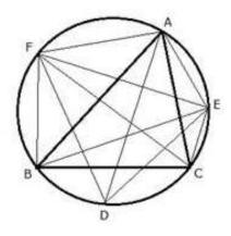
Join ED, EF and DF. Also join BF, FA, AE and EC.
